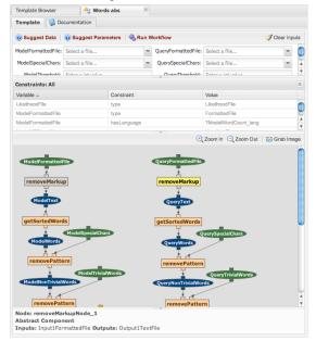
The component removeMarkup is a class of components that includes two executables: html2text and pdf2text. Depending on what kind of data is input to the workflow, the appropriate executable will be selected.
