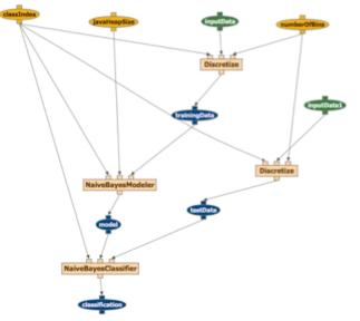
Figure 1. A workflow that discretizes datasets, then creates a model to classify test data. Semantic constraints are shown at the top, stating properties of workflow constituents such as software components and intermediate data. The dataflow is shown graphically at the bottom.
