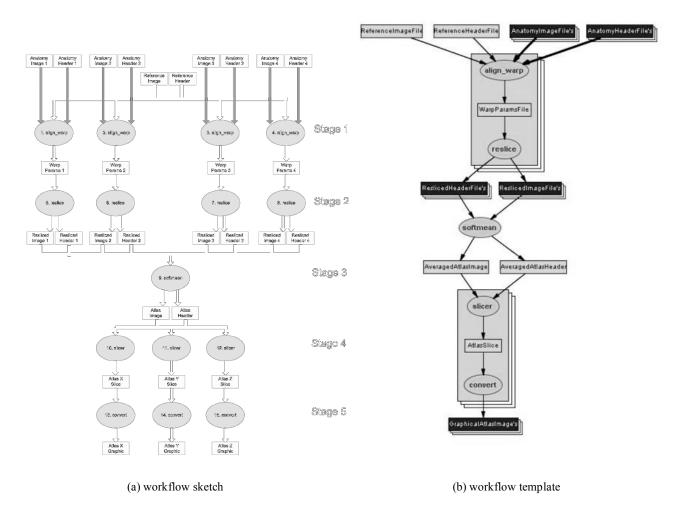
Figure 1: In our layered workflow design approach, users design a *workflow sketch* and from it create a formal model of the components and their data flow in a *workflow template*.
