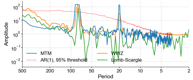
Figure 2: Spectral density for a synthetic timeseries with prescribed periods of 20 and 80, a polynomial trend of order 2, a white noise/signal ratio of 0.5, 40% missing values, and outliers 5 to 7 standard deviation away from the mean using MTM, WWZ and Lomb-Scargle methods.
