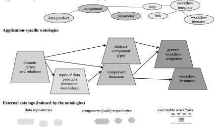
Fig. 1.5. Semantic workflow representations include application-specific ontologies organized as specializations of generic application-independent definitions. The ontologies can be used to index repositories of data, components, and executed workflows.
