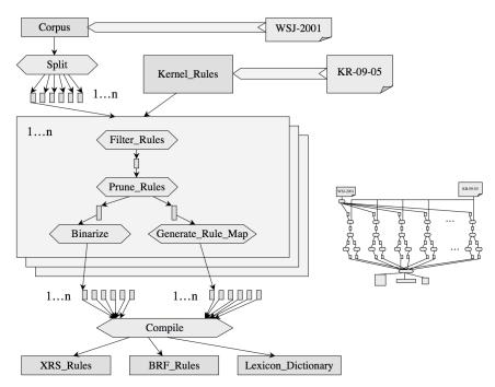
Fig. 1.3. A workflow instance specifies the data to be processed by a workflow template in an execution-independent representation.
